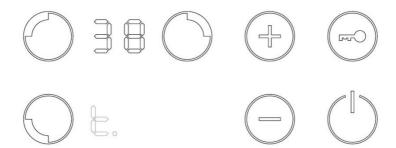
When the timer is waiting a time selection, the timer value can be selected between 0 and 99 minutes touching the + or - keys. The remaining time will be displayed in the opposite part of timed heater.
