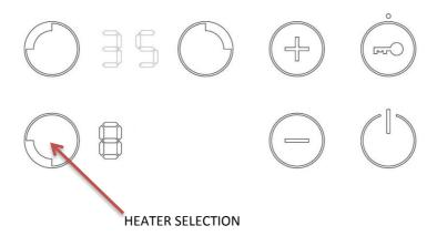
A heater is selected by touching the heater [HEATER\_SELECTION] key for 500 milliseconds, a beep sounds and the heater display shows the power level with normal brightness.
