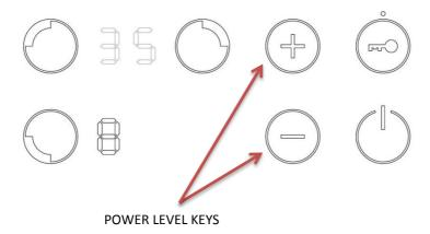
With the heater at power level 0, the - key raises the cooking level to 9.
